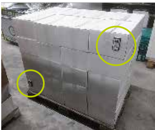
Positioning of outside loggers on the pallet
