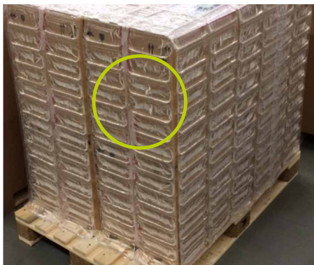
Positioning of inside logger inside the cardboard box
